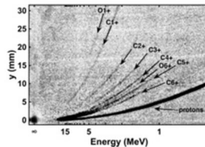
**Fig.2.** Measurement of emitted ion spectra obtained using Thomson parabola. Traces of H<sup>+</sup>, C1<sup>+</sup>– C6<sup>+</sup>, O1<sup>+</sup> and O6<sup>+</sup> ions are marked according to calculations of ion trajectories. Proton energy is laid off on the horizontal axis
