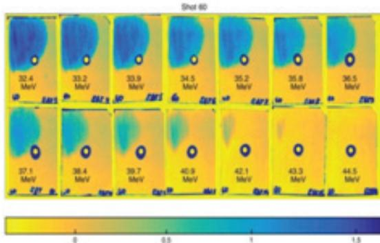
**Fig.1.** Radiochromic films exposed to a record proton beam accelerated by 7J laser pulse. The depicted energies correspond to the proton Bragg peak in energy deposition for a sensitive layer of particular film. Maximum proton energy is 43.3 MeV.
