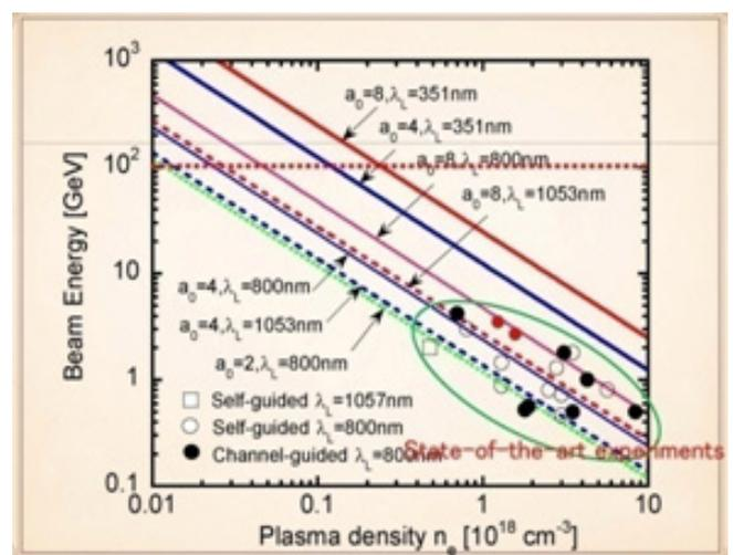
Fig. 2. Current experimental data for beam energy vs. plasma density
